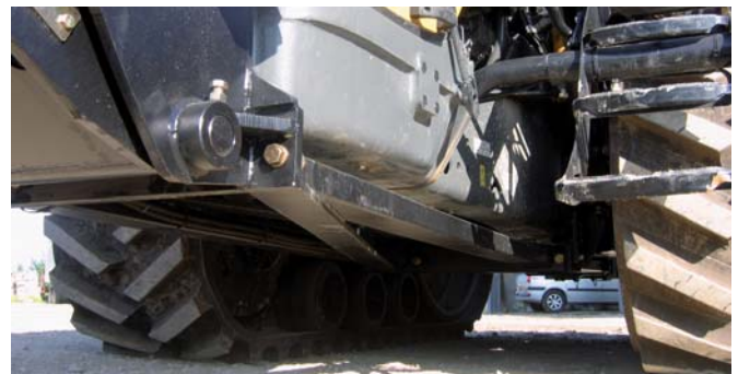
The lower reinforcing frame maintains crop clearance
