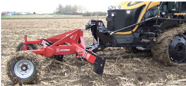
HDIT front hitch with optional DYNA CONTOUR® attached to a UNIPASS® front sub-soiler
